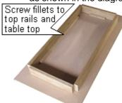
Next, lay the 4 fillets (e) in place against the top rails (b) and the underside of the table top (c). Screw through the fillets (e) into the table top (c) and then screw through the fillets (e) into the top rails (b). Sometimes it might be easier to pre-drill the screw holes through the fillets.
